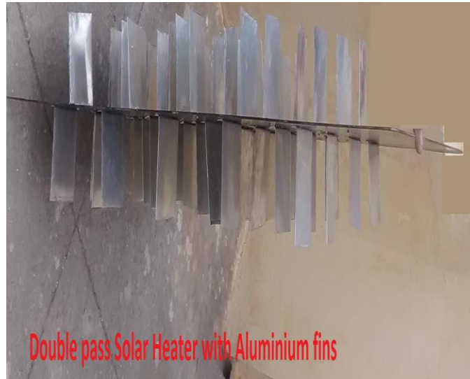
FIGURE 2. double pass solar heater with aluminum fins
