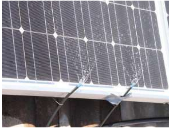
FIGURE 10. Solar Setup Including Water Cooling
