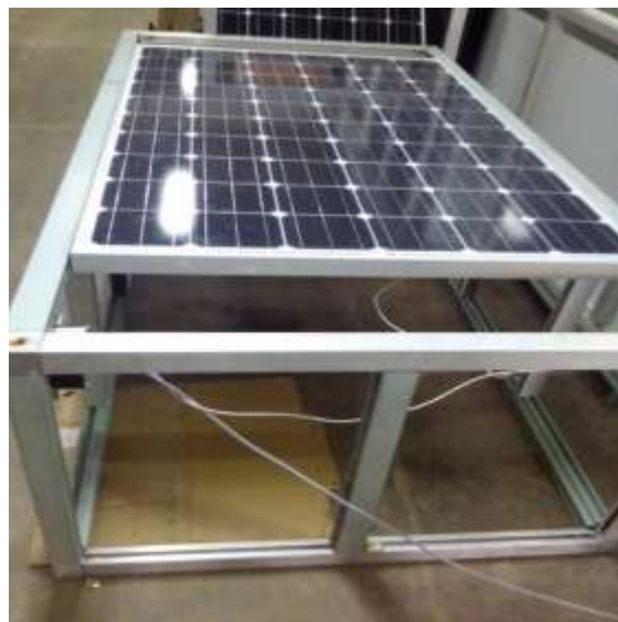
FIGURE 4. PV system using anti-reflection coating
