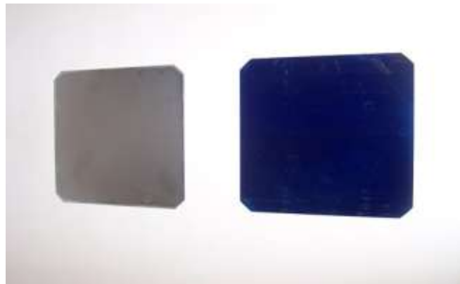
FIGURE 2. Photograph of Non-AR coated and AR Coated Silicon wafer
