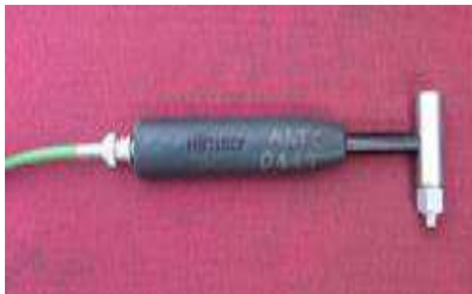
FIGURE 4. Impact hammer with metal tip
