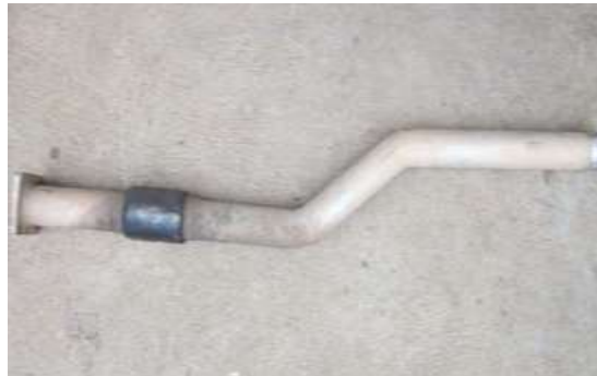
FIGURE 2. Vehicle A second pipe in exhaust system taken for modal testing
