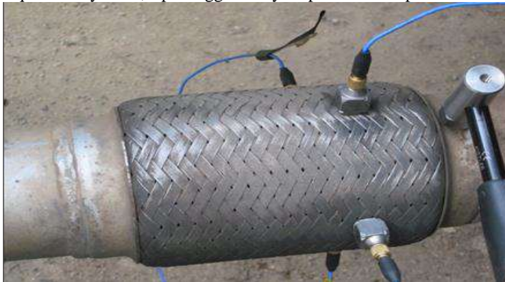
FIGURE 5. Impact testing of the flex bellow component
