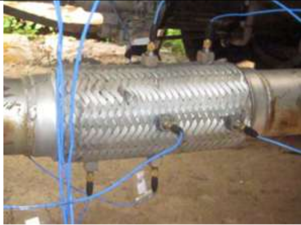
FIGURE 14. Acceleration positions on the flex bellow component
