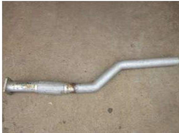
FIGURE 13. Vehicle A second pipe with new flex bellow in exhaust system taken for modal testing
