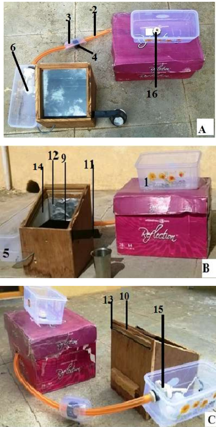
FIGURE 2. Working model of solar distillation system
