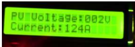
FIGURE 8. Minimum voltage produced at100W/m 2 condition
