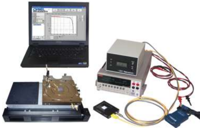
FIGURE 2.PV module performance monitoring using graphical user interface
