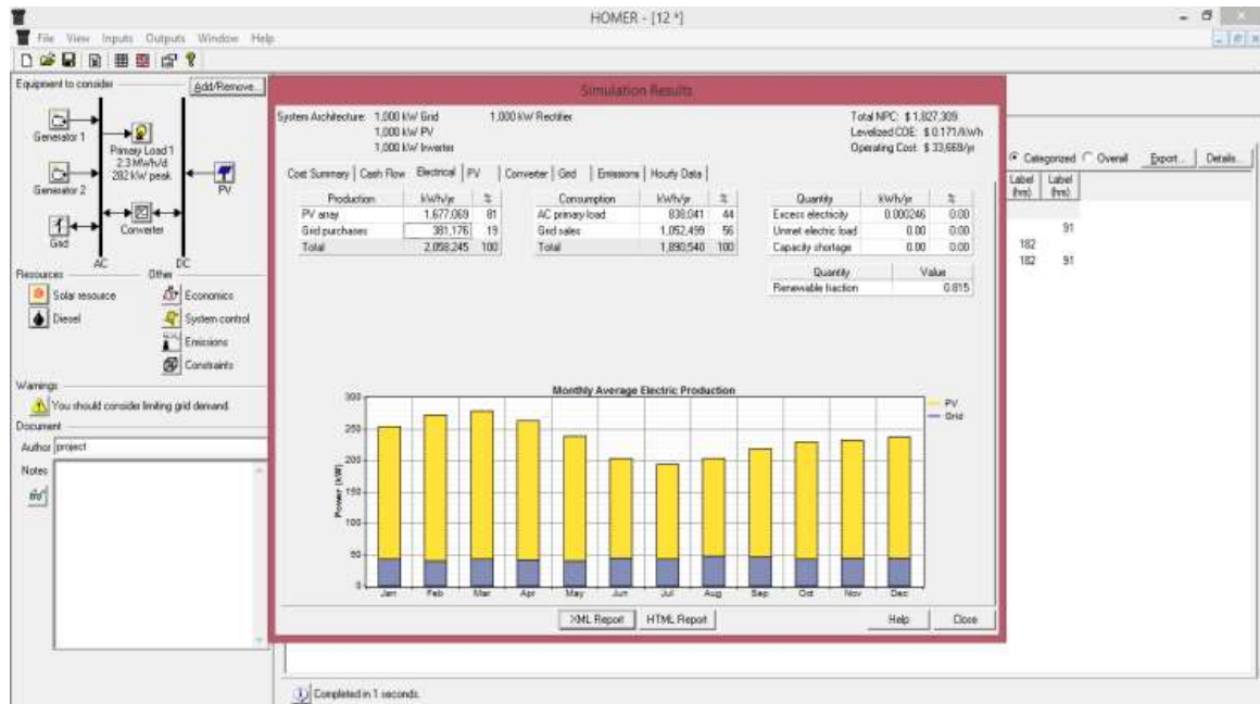
FIGURE 6. Load Sharing Between PV and Grid
