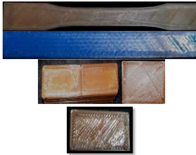
FIGURE 6. Tensile, Flexural, Compression, Hardness and Impact samples used in the study
