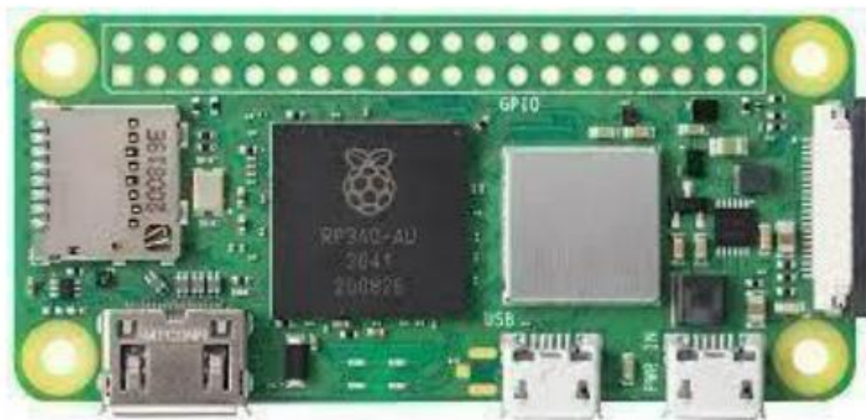
FIGURE 4. Raspberry Pi Zero 2W specification
