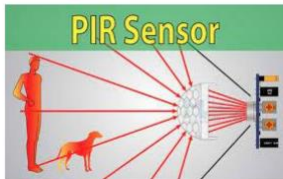
FIGURE 11. PIR Sensor Working Model
