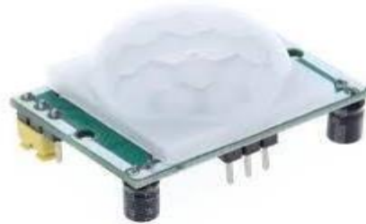
FIGURE 10. PIR Sensor (Passive Infrared Sensor)
