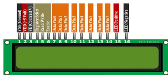
FIGURE 1. 16*2 LCD Module Pin out
