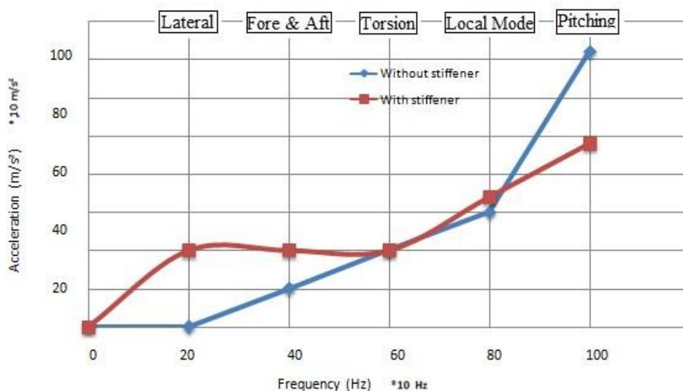
FIGURE 6. Acceleration Response Plot – Node 2
