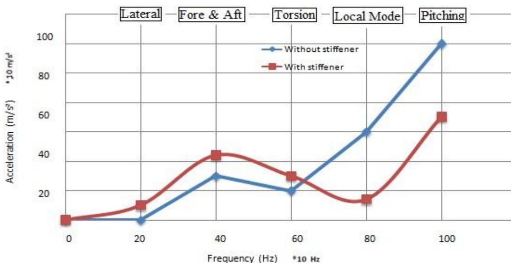
FIGURE 7. Acceleration Response Plot – Node 3
