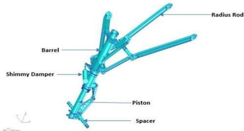
FIGURE 1. Nose Landing Gear Assembly
