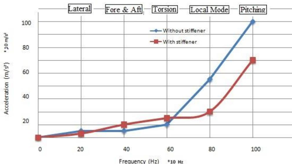
FIGURE 8. Acceleration Response Plot – Node 4
