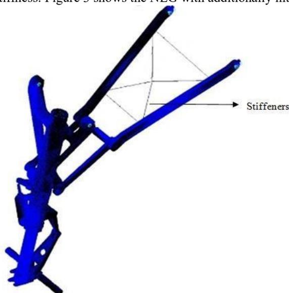
FIGURE 3. NLG with Additionally Introduced Stiffeners
