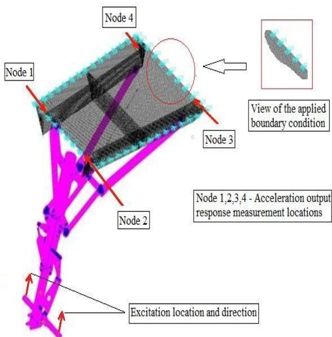
FIGURE 2. Finite Element Model of Landing gear with Floor Attachment
