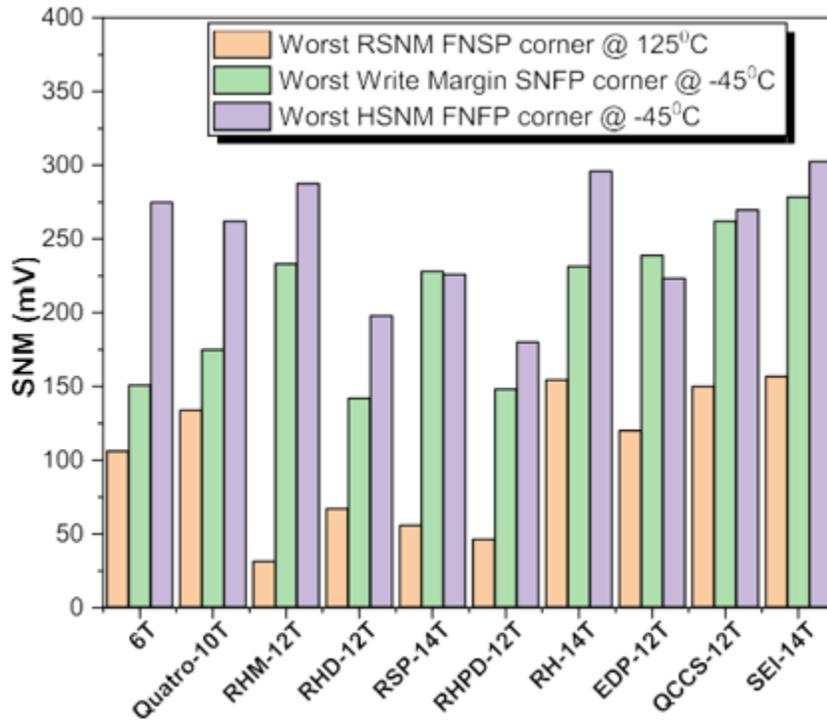
FIGURE 5. Comparison of stability and temperature analysis of all memory cells in the worst case.
