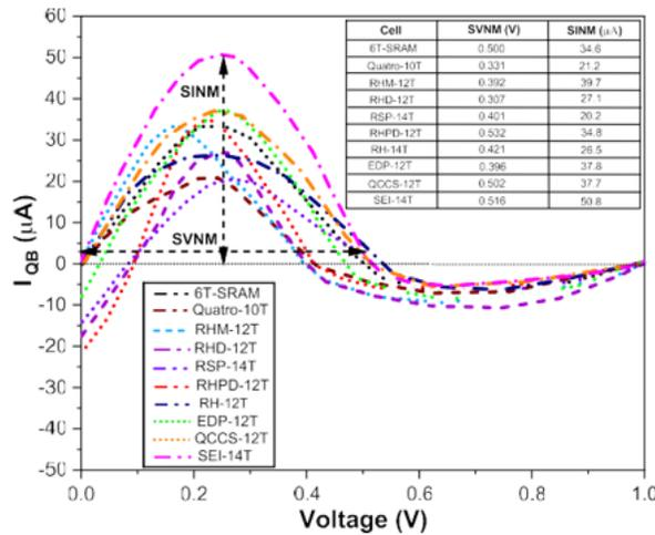
FIGURE 6. N-curve comparison of existing and proposed memory cells.
