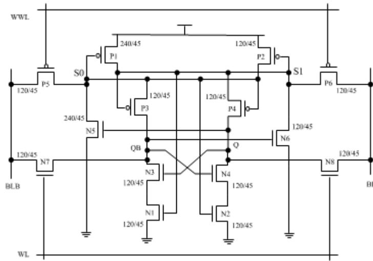
FIGURE 3. SEI-14T memory cell schematic diagram.
