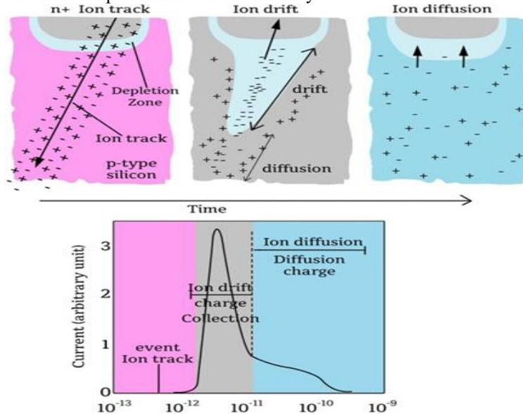
FIGURE 1. High-energy particle impact, ion footprint, and transient pulse generation.
