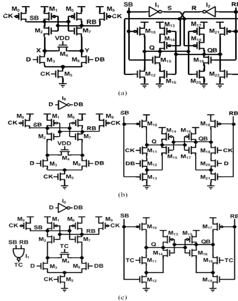
FIGURE 4. Flip-flops utilizing sense amplifiers: (a) Nicholas' SAFF [17], (b) Stroll's SAFF [18], and (c) SAFF-TCD [19].
