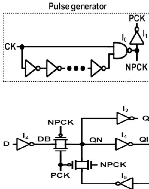
FIGURE 2. Flip-flops based on pulsed latches: TGPL
