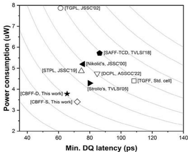
**FIGURE 11.** Minimum DQ delay and power consumption of single-ended (empty) and differential (filled) flip-flops under 0.1 input TT corner operation, with a 1-V supply voltage and a temperature of 27°C
