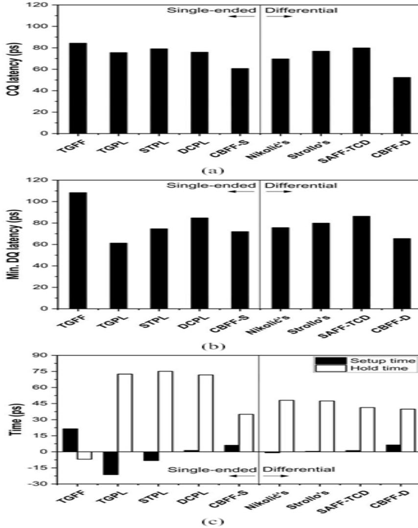
FIGURE 9. Timing performance of flip-flops: (a) CQ delay, (b) minimum DQ delay, and (c) setup and hold times at the TT corner, with a 1-V supply voltage and a temperature of 27°C
