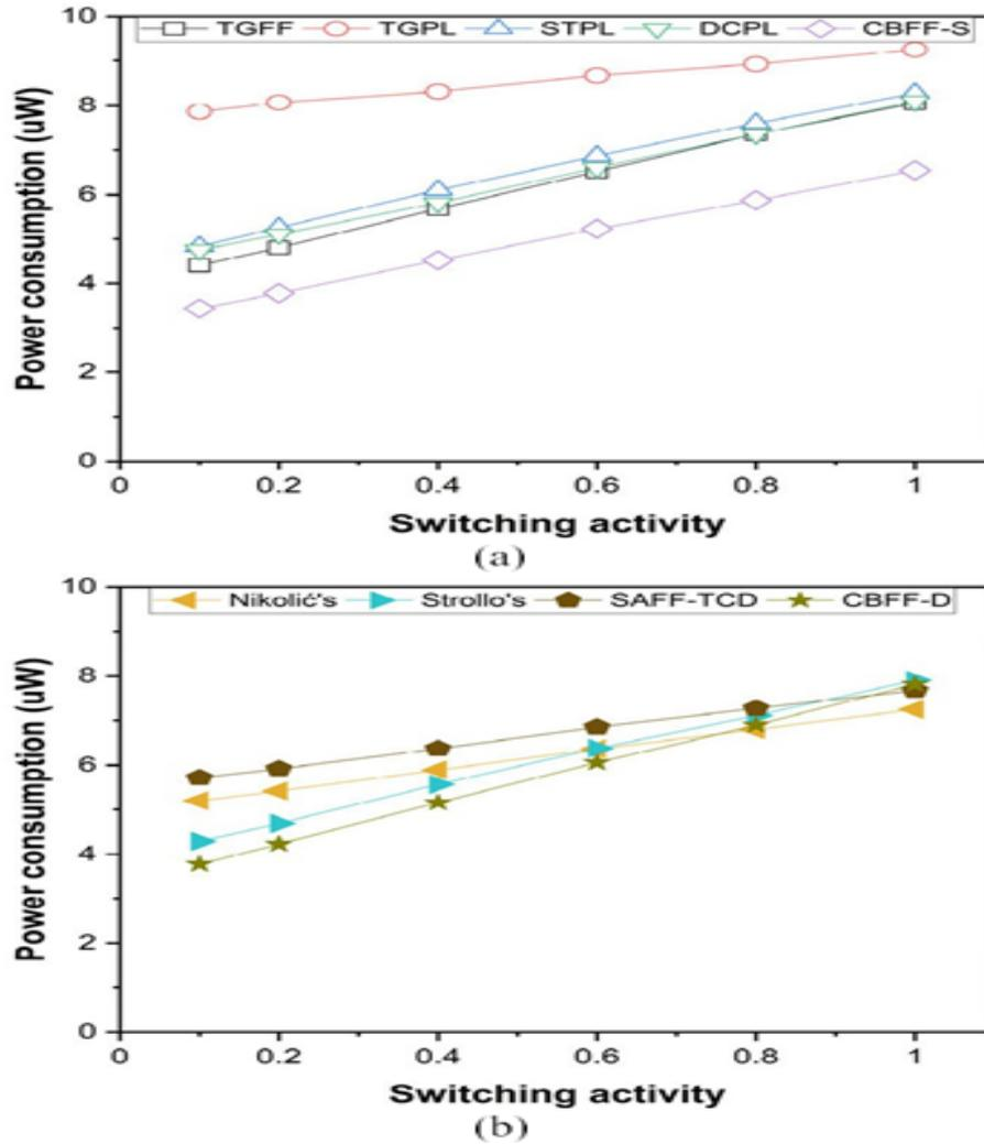
**FIGURE 8.** Input switching operation and Power consumption for (a) single-ended and (b) differential flip-flops at the TT corner, with a 1-V supply voltage and a temperature of 27°C.
