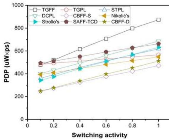
FIGURE 10. Input switching function and power-delay product (PDP) of TT corner flip-flops with a 1-V supply voltage and a temperature of 27°C
