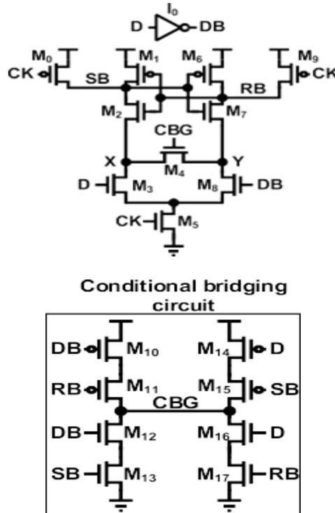
FIGURE 5. Sense amplifier stage incorporating a conditional bridge circuit
