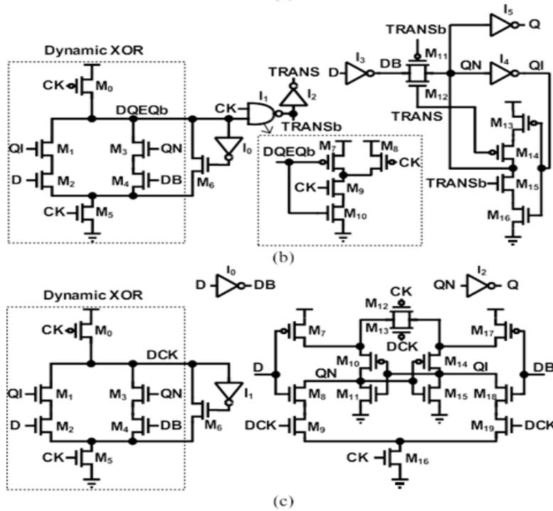
FIGURE 3. Flip-flops based on pulsed latches: (b) STPL and (c) DCP.
