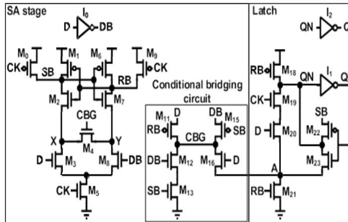
FIGURE 6. Single-ended variant of the proposed flip-flop
