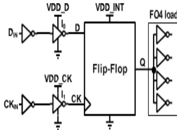
FIGURE 7. Flip-flop simulation environment.
