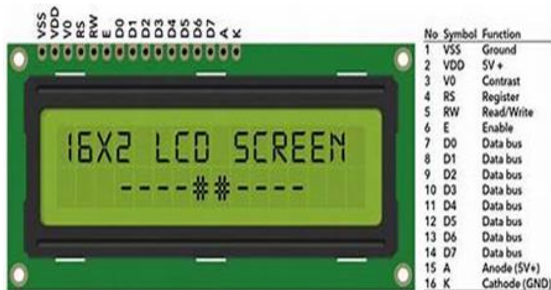
FIGURE 7. Pin Diagram of LCD
