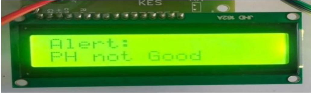
FIGURE 6. LCD Display of LoRa Receiver
