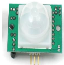
FIGURE 3. PIR Motion Sensor (Passive Infrared Sensor)
