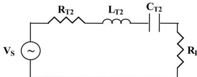
FIGURE 3. Electrical circuit representing a drone. The resistance  $R_D$  is the drone equivalent resistance appearing from the
