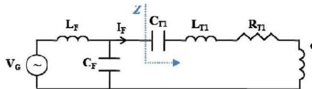
Fig.2. Electrical circuit representing a pad.
