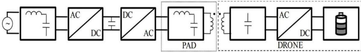
FIGURE 1. Recharge system. Only one pad-drone couple is represented in the figure. All pads are connected in parallel.
