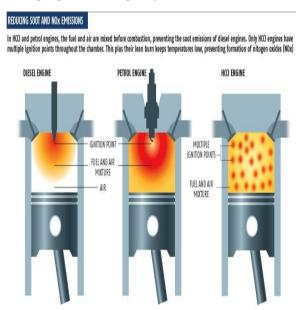
Conventional Diesel engines can be converted to run in the HCCI mode. The intake air should be preheated with an air heater. As of today, various fuels such as propane, butane and methane have been tested on HCCI engine
