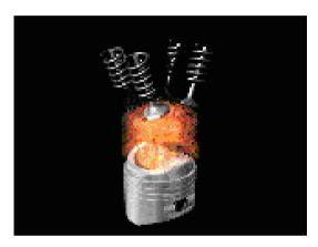
The required control system is fundamentally more challenging than conventional engines because the ignition is sensitive to very small changes in temperature. When a load is suddenly added, as when a vehicle goes from idle to cruising speed, the control system must adjust the temperature, pressure and composition rapidly enough to maintain stable combustion. Several approaches have been suggested for combustion control in HCCI Engine, They are
