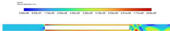
FIGURE 6. Cuboidal nose profile pod - velocity contours
