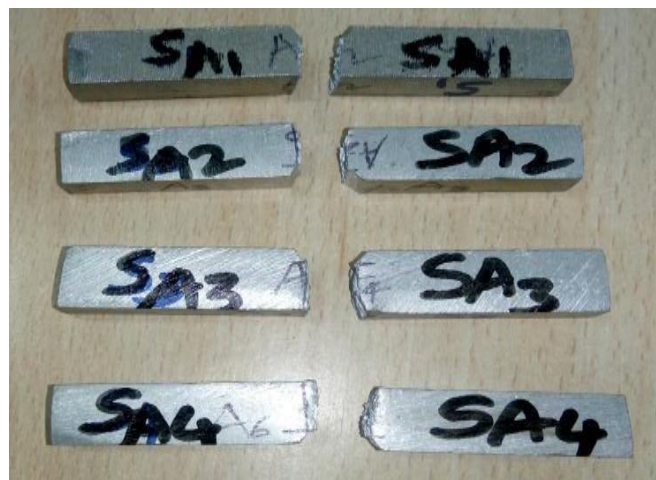
FIGURE 5. Impact strength tested specimen of Al6063/ B 4 C composites
