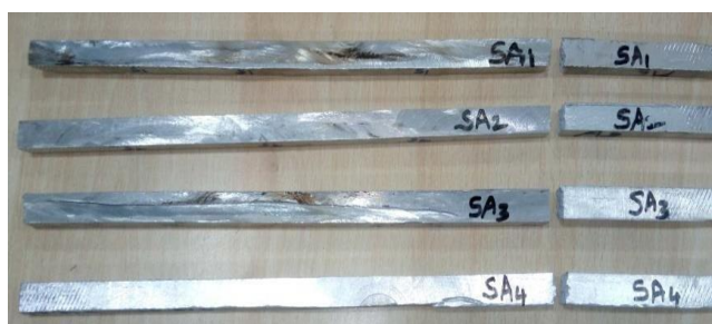
FIGURE 3. Tensile tested specimen of Al6063/ B4C composites
