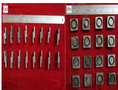
FIGURE 1. Bonded specimens were photographed for (a) Lap Shear test (b) Ram Tensile test
