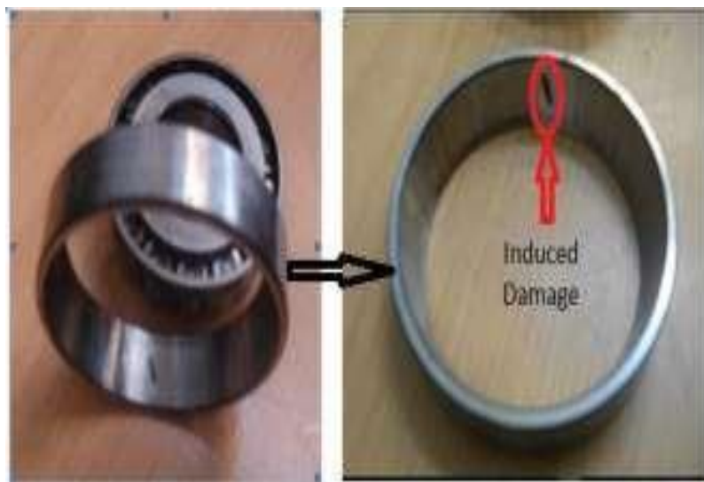
FIGURE 3. Seeded damage on outer race of a bearing.
