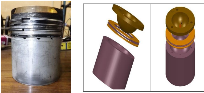
FIGURE 2. Photo Graphic View of Aluminum Piston with Brass Crown and Air Insulation
