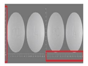
Prepare a binary threes hold image with to establish the size of the query pill (logical 0). Because the graph scales in the pill picture collection are already white, a high threes hold of 0.90 is found to be sufficient. The height and width of the pill are then calculated using the connected components of the threshold binary picture component have a value other than 1. The
