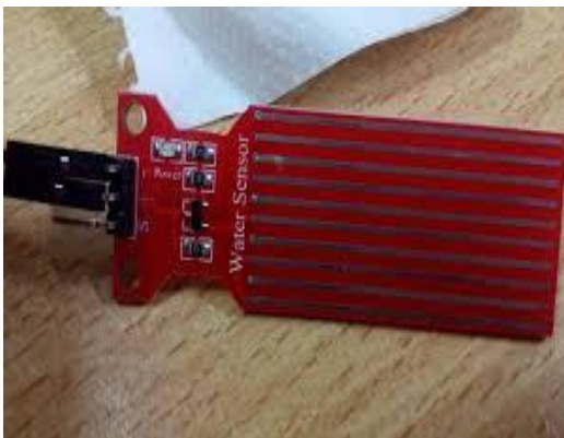
FIGURE 4. Water Level Indicator Module FIGURE 5. Temperature Sensor Module
