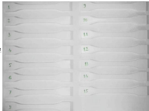
(A) (B) Fig. 1.3. (A) ASTM D-638 standard (B) 3D printed Specimens as per standard
