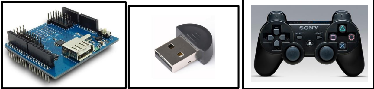
USB Host Shield; USB Bluetooth Dongle; Sony PlayStation Controller (Wireless)
