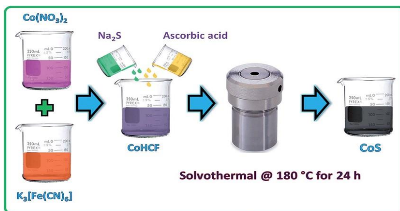
Figure 1: Schematic representation of solvothermal process of synthesis of nanomaterials
