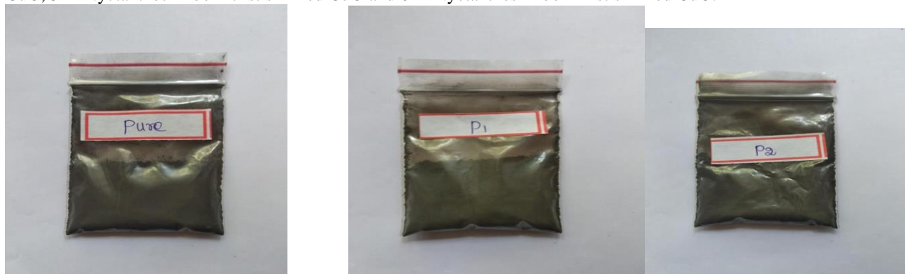
Fig 3.1: pure CuO nanoparticle Fig3.2:3ml Nyctanthes Arbor-tristis mixed CuO; Fig 3.3: 6ml Nyctanthes Arbor – tristis mixed CuO
