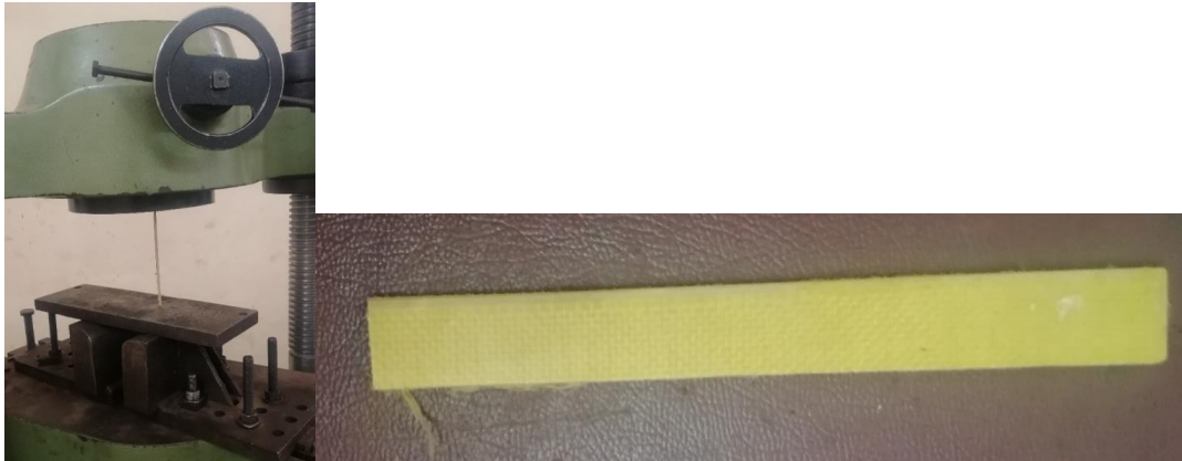
Figure 8. Compression Test Setup; Figure 9. Compression Test Specimen
