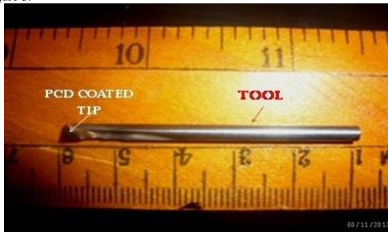
Figure.3. Solid carbide tool coated with PCD at tip.
