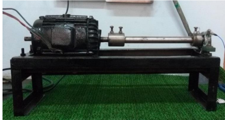
Fig. 1 The Test Rig to measure the vibration signature of the shaft mounted.
