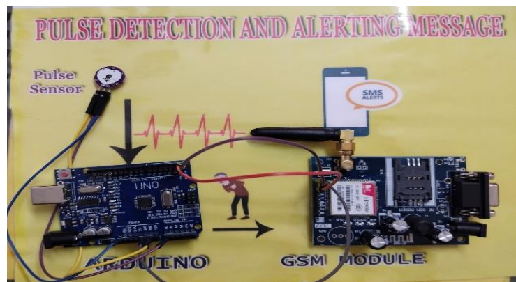
FIGURE 1. Heart pulse rate detection and alerting using Arduino with GSM module
