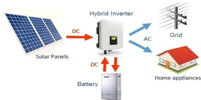
FIGURE 4. Basic layout diagram of a common solar hybrid system
