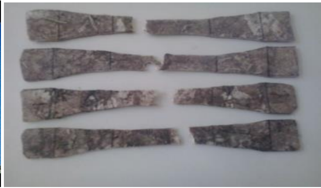
Figure 3.2. Tensile test specimen of cactus
